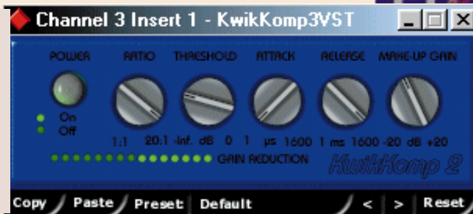
▶ FIG 3 KWIKKOMP IS AN ANALOGUE-STYLE COMPRESSOR OFFERING RATIO, THRESHOLD, ATTACK, DECAY AND GAIN MAKE-UP PARAMETERS. IT'S EASY TO USE AND CAN ADD A LOT OF PUNCH TO INDIVIDUAL DRUM SOUNDS
